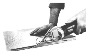
flush trimming of projecting edges with side guide
