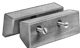
set of blocks, for straight cutting of corrugated plastics
