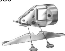
assembling side guide with two wing screws
